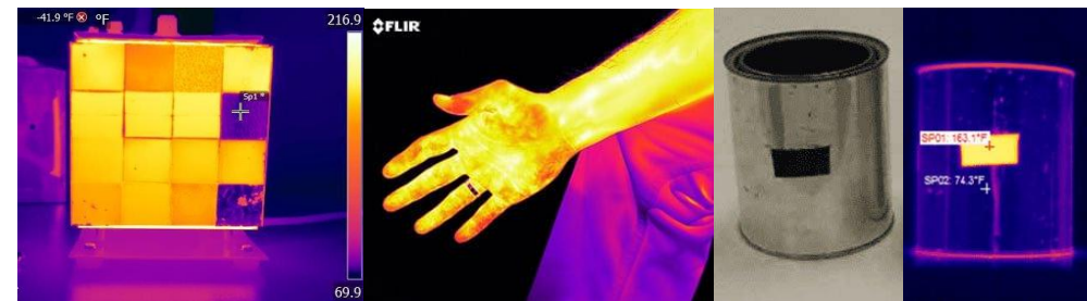
Same Temp. Diff. Emissivity Same Temp. Diff. Reflectivity Processing for Temp. Measurement
